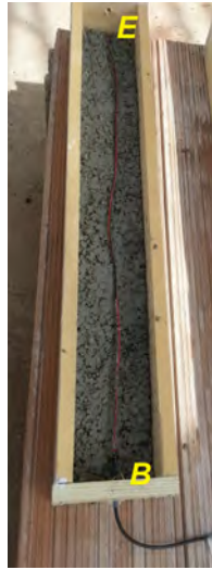
Figure 3. Preparation of the concrete sample, with the embedding of SE1.
