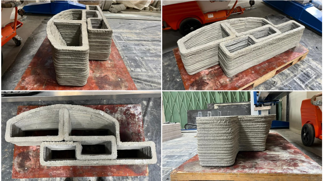
Fig. 42 Perspectives of the reverse printed component in its utilization position (after one month of setting).
