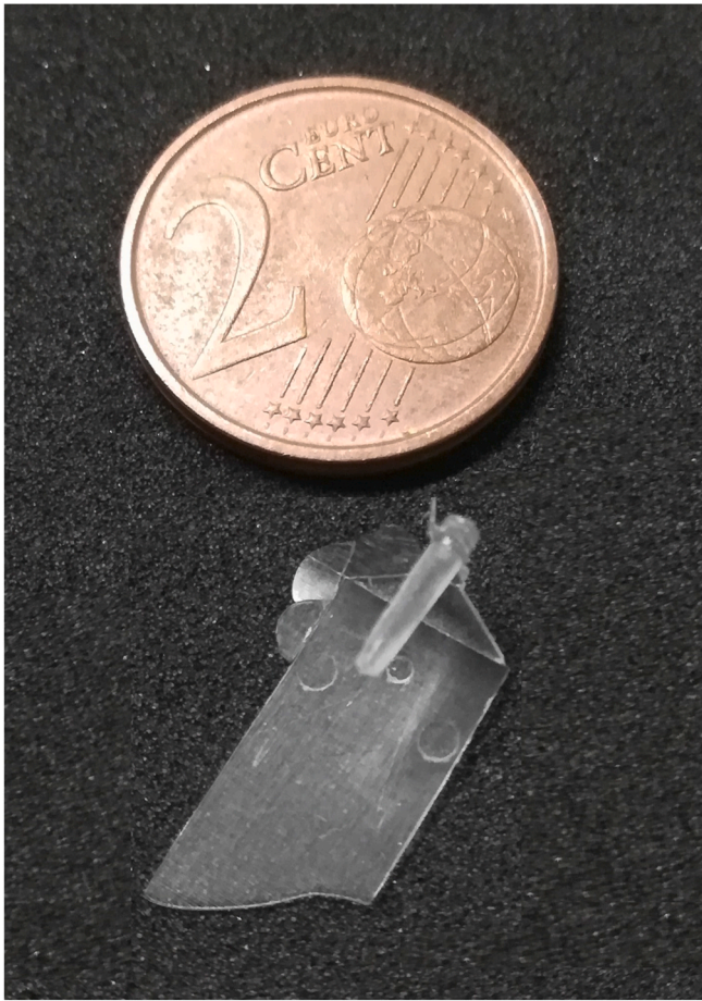
Fig. 7. Example of incomplete filling and burr on test parts in PMMA of 100 \mu\text{m} thickness.
