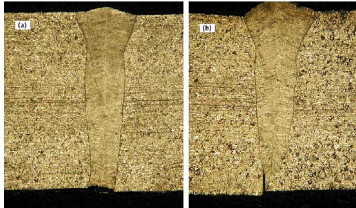
Figure 6. Macrographs of the joint cross sections: (a) full penetration: P = 1.8 kW, v = 80 mm/s, Q_{\text{He}} = 100 L/min (zone 1); (b) partial penetration: P = 1.0 kW, v = 80 mm/s, Q_{\text{He}} = 100 L/min (zone 3).
