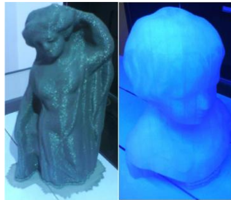
Fig. 12. Production with low cost 3D printer (FDM techniques) of scanned objects
