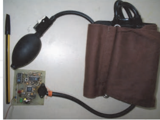
Fig. 29. Prototype of the arterial pressure measurement instrument, PC-based and wi fi connected to PC
