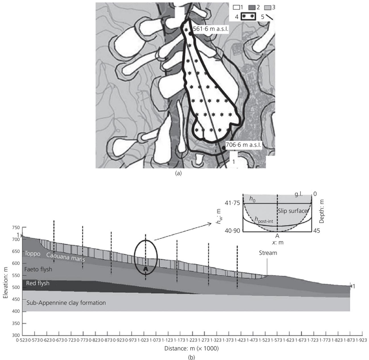
**Fig. 7.** (a) Geomorphological map of the Volturino unstable slope (modified from Lollino *et al.*, 2010): 1 – sub-Appennine clays, 2 – Toppo Capuana marls, 3 – red flysch, 4 – landslide of reference in the paper, 5 – trace of the section considered in the LE analyses; (b) longitudinal section of the landslide body subjected to LE analysis with the prototype scheme of the transverse section of reference in the seepage analyses
