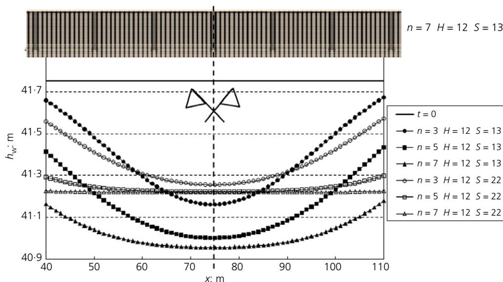
Fig. 6. Details of the finite-element mesh adopted for the seepage analysis and curves of pressure head calculated for different trench systems at depth  $z = 45$  m from g.l., after 5 years of transient seepage
