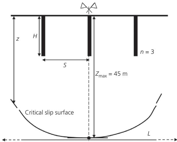
**Fig. 4.** Schematic cross-section of the drainage system and of the slip surface.  $S$  – spacing between trenches;  $H$  – depth of trenches;  $z$  – depth of slip surface;  $L$  – total width of the trench system
