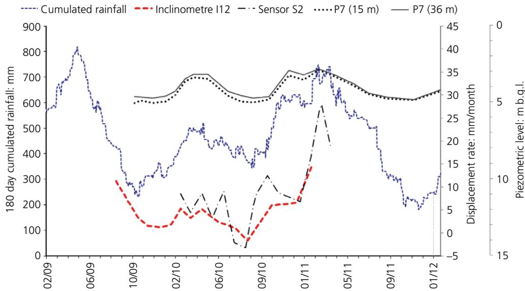
**Fig. 3.** Rate of movements measured with GPS sensor S2 and inclinometer I12 (at 19 m depth); piezometric levels logged by means of the P7 electric pore pressure cells (at 15 and 36 m from g.l.) and 180 days cumulated rainfalls at Pisciolio site (Cotecchia *et al.*, 2014a)
