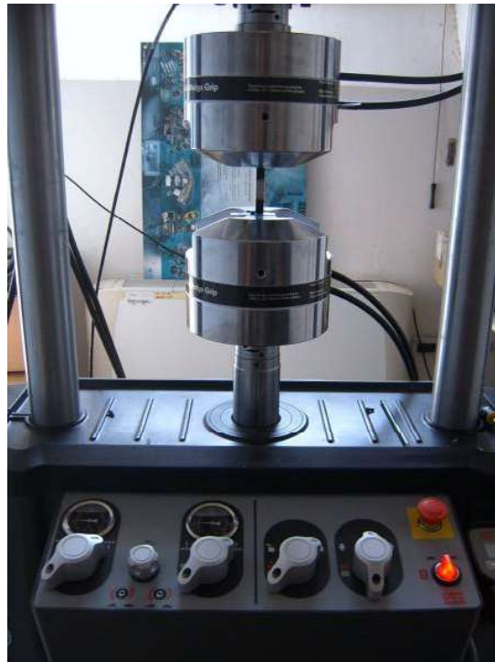
Figure 6. Setup of tensile test.
