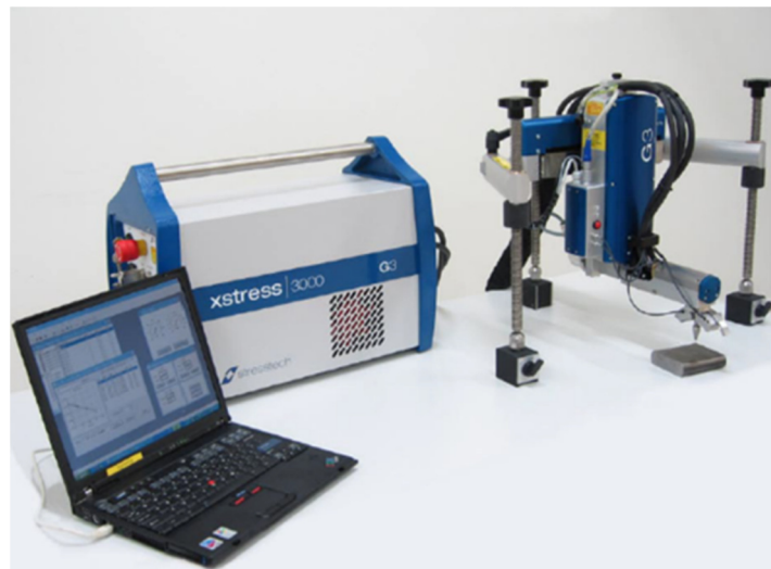
Figure 2.8 Example of commercial diffractometer for residual stress measurements
