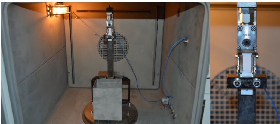
Figure 8.13 An example of specimen mounted in the grips in the temperature-controlled chamber
