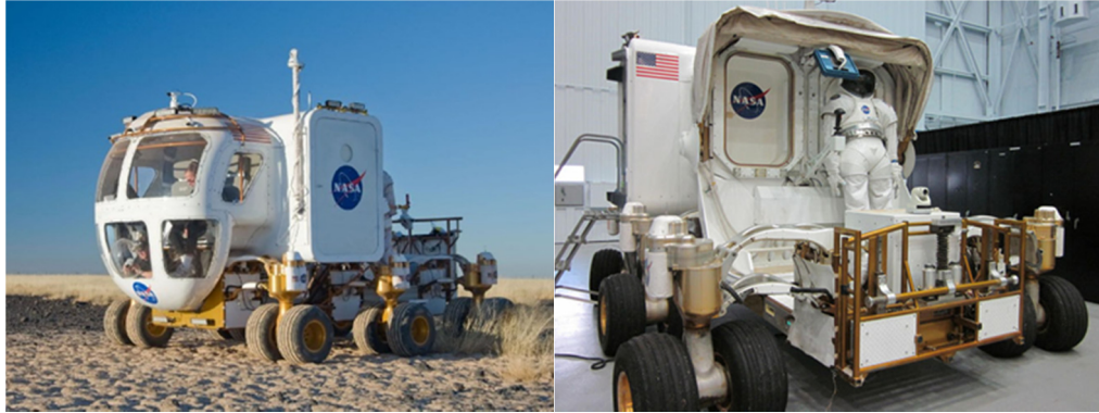
Figure 7.9 More than 70 parts of the NASA rover has been made using FDM
