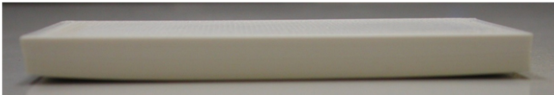
Figure 7.12 Warpage of the FDM part
