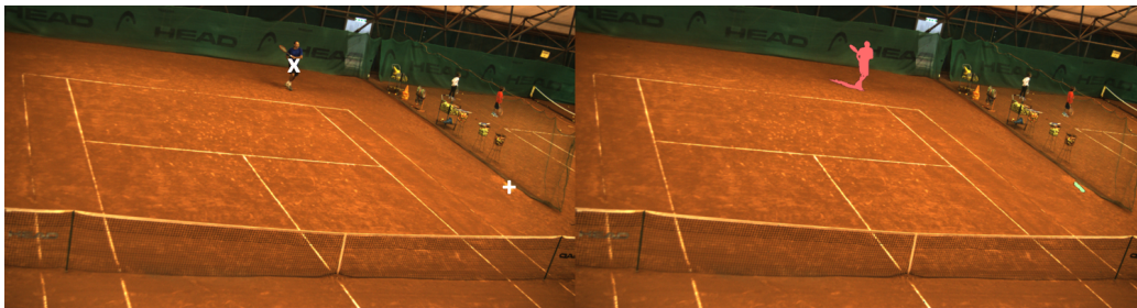
Figure 6.4: Graphical output of the low level processing in terms of entities coordinates and player silhouette. On the left side, two different symbols are used to mark the entities: X for the player and + for the ball. On the right side, the silhouette of the player is highlighted in red and ball in green. Data from this stage is essential to reconstruct three dimensional coordinates and proceed with the analysis of the match performing the subsequent tasks.
