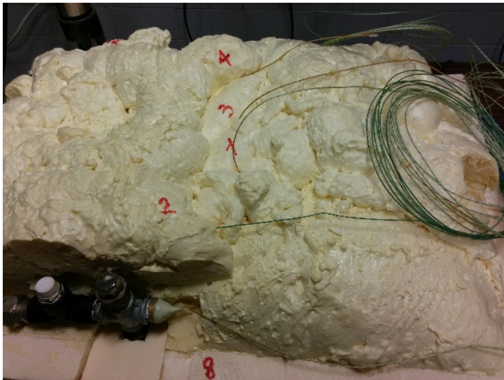
Figure 46 Particular of thermal insulate fractured limestone block.
