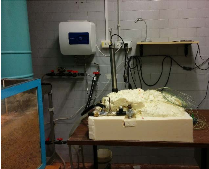
Figure 45 Thermal insulate fractured limestone block
