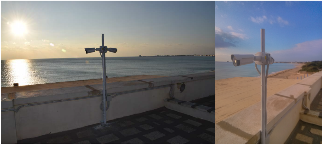
Figure 3.7 Right: Cameras location in Torre Lapillo (TL); Left: Cameras installation and the NW coastal stretch monitored.
