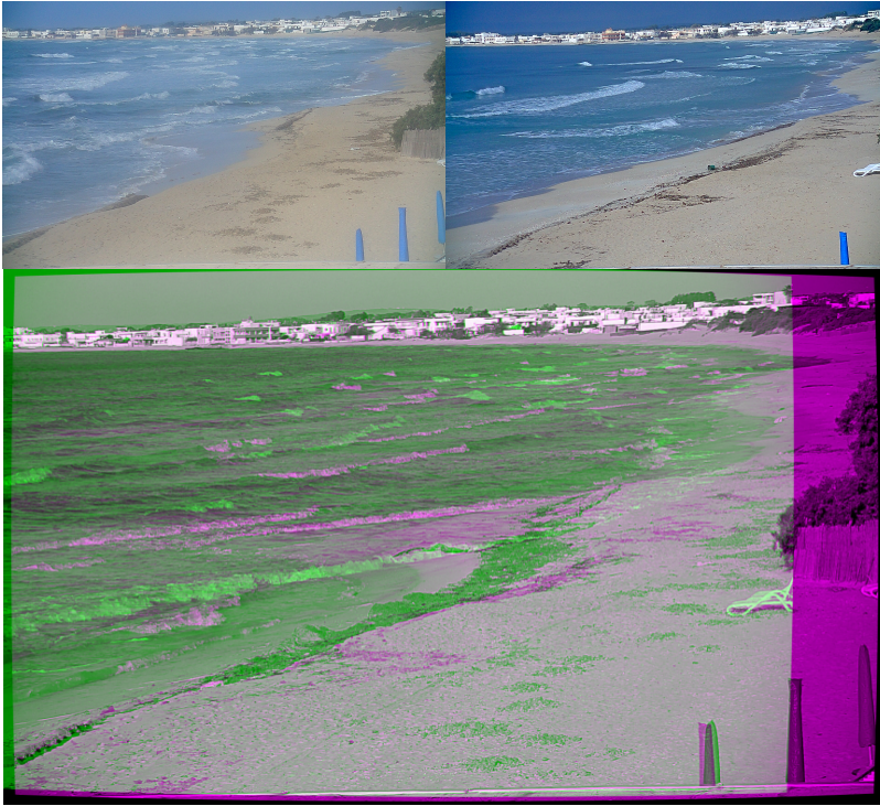
Figure 3.11 Top left: Original image at the time of external calibration; Top right: Image displaced; Bottom: Overlay of original registered image over displaced one, by using alpha blending, showing high accuracy (green channel).
