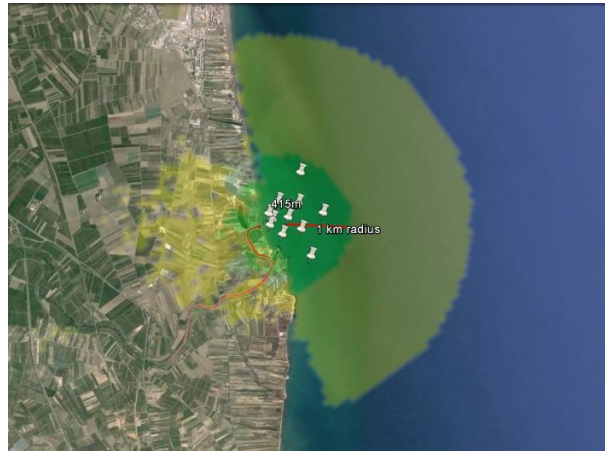
Fig. 24 Coverage simulation around central buoy (“415m” in Fig. 10): green zone has strong signal (Link Margin > 10 dB), yellow zone has weak signal (Link Margin < 10 dB)
