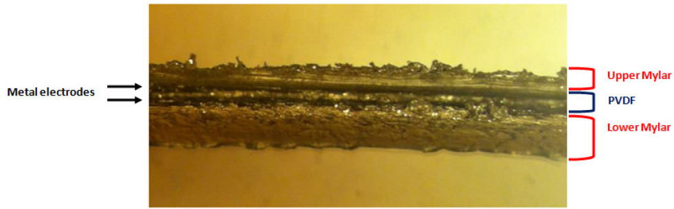
Figure 4.31 - Longitudinal section of cantilever beam, observed under a microscope.
