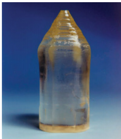
Figure 1.5 - Kistler's PiezoStar: Ø55 [mm], weight 1.8 [Kg] (Courtesy to Kistler Group).
