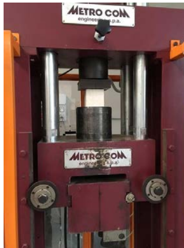
Fig. 8. Evaluation of compression strength of an ashlar.
