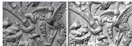
Fig. 11. Same detail of the polygonal model obtained with the PSA laser system (left) and with the DCRP system (right).
