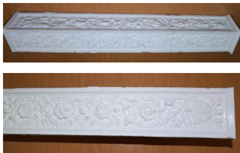
Fig. 12. Down scaled column copy fabricated by additive manufacturing.
