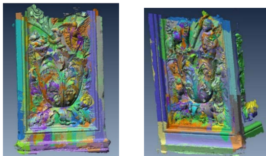
Fig. 3. The two point clouds, one for each lateral face, obtained using the PMA with laser scanner.
