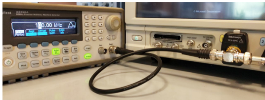
(b) TDR setup with an Arbitrary Waveform Generator (pulse signal with \sim 10\text{ns} width) and an oscilloscope channel
