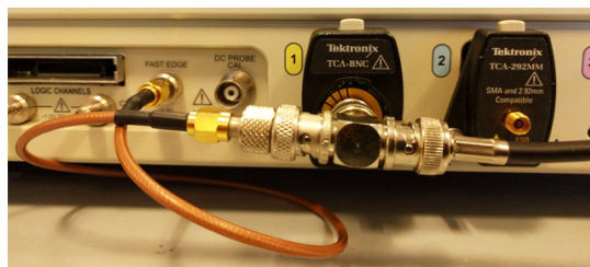
(c) TDR setup with a fast edge ( \sim 200\text{ ps} rise time) generator and an oscilloscope channel
