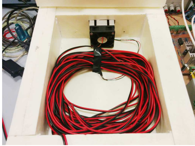
FIGURE 2.5: Positioning of the bi-wire in the thermally-controlled box (TCB).
