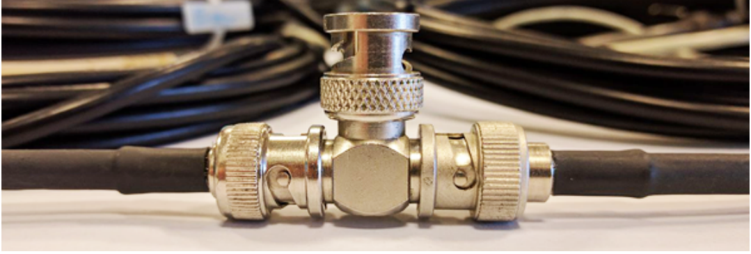
FIGURE 6.10: Junction between 5 m long RG58-CU coaxial cables
