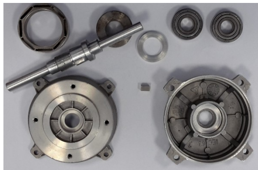
fig. 60: Flanges IEC 63, bearings, shaft, rotor
