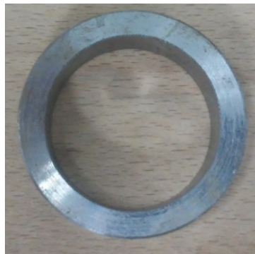
fig. 83: Dummy rotor in stainless steel, used to estimate the mechanical losses
