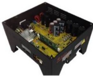
fig. 162: High voltage motor control
