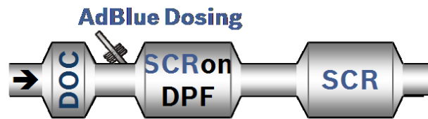
Figure 2.7 After-treatment layout for the test bench activity
