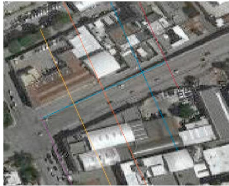
Fig. 4. Construction of virtual sections for the two-lane road.
