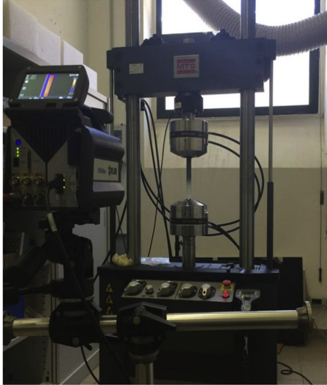
Figure 1. Experimental set-up adopted for thermographic tests.
