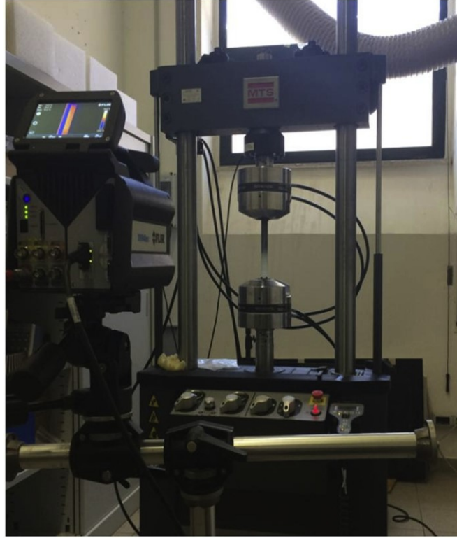
Figure 1. Experimental set-up adopted for thermographic tests.
