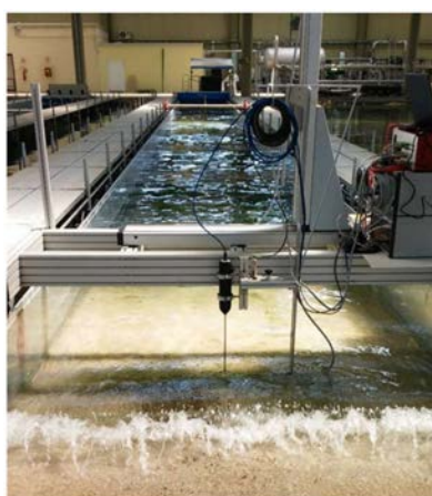
Figure 1. Frontal view of the wave channel in the Coastal Engineering Laboratory (LIC) of the Polytechnic University of Bari. The array with the measurement instrumentations is in the foreground.
