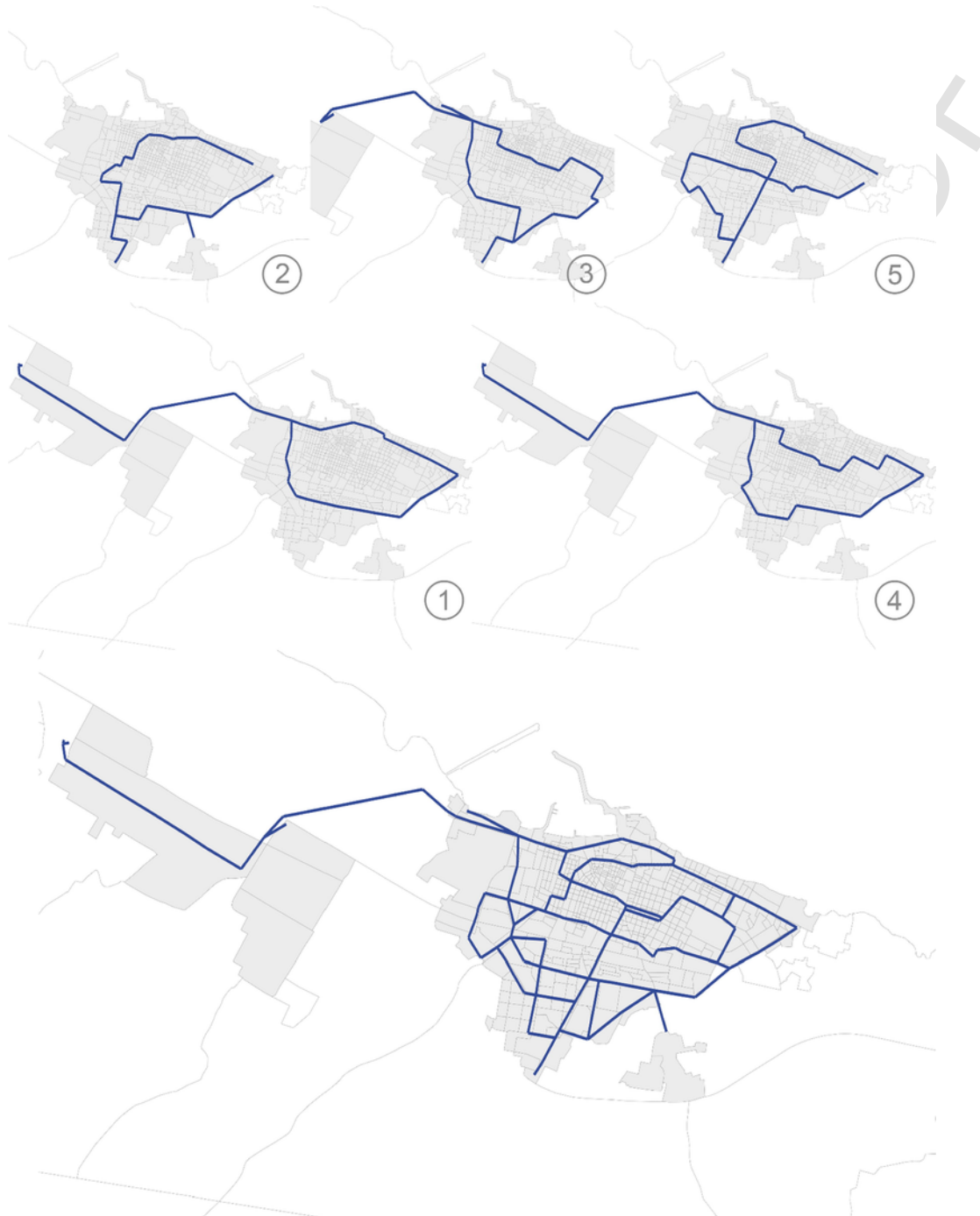
Fig. 8. Path covered by each one of the optimal routes, and by the optimal transit route set as a whole.
