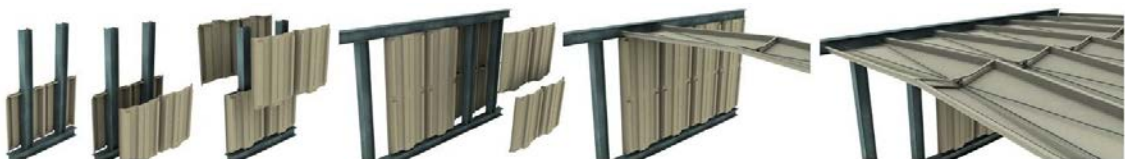
Fig. 5. Geometry and assembling scheme of wall shells.
