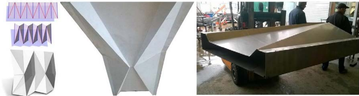
Fig. 2. Design and prototyping of roof elements.
