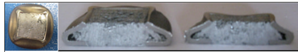
FIGURE 23: Example of a steel tube filled with aluminium foams cut after compressive test.
