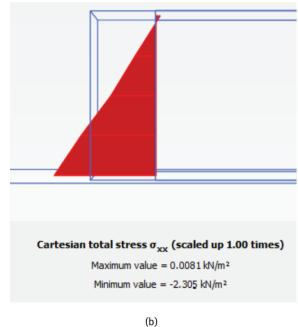
**Figure 3:** Total horizontal stress  $\sigma_{\omega}$ : (a) Prototype; (b) Scaled model. (Plaxis notation for the sign).
