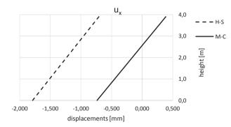
Figure 4: Effect on the predicted prototype behavior of two constitutive models (Mohr-Coulomb and Hardening Soil): results are shown in terms of displacements along x-direction (u).
