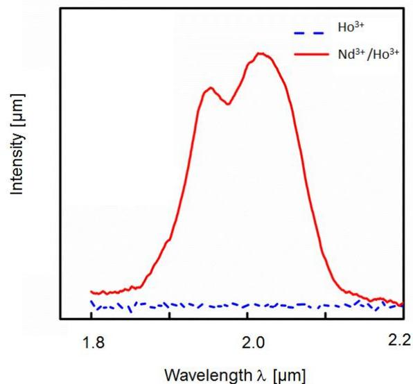
**Figure 1.** Emission spectra of Ho<sup>3+</sup> and Nd<sup>3+</sup>/Ho<sup>3+</sup> co-doped tungsten tellurite glasses. Figure adapted from [18].
