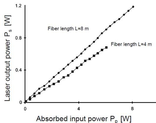
**Figure 5.** Characteristics of the  $\text{Er}^{3+}$ -doped fluoride glass fiber laser [25]. Figure adapted from [25].
