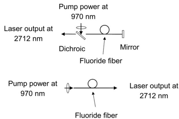
**Figure 4.** Set-ups of the two fiber laser configurations demonstrated in [25]. Figure adapted from [25].
