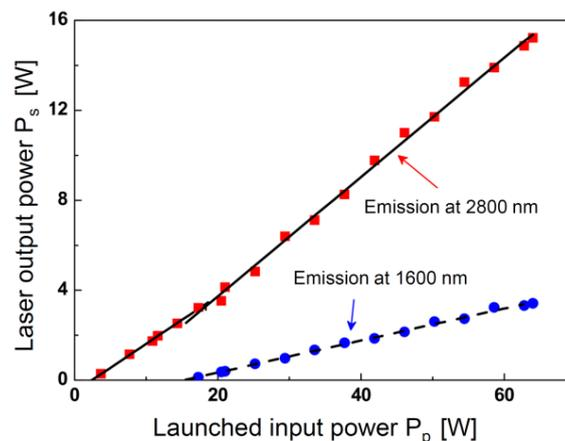
**Figure 7.** Characteristics of the fluoride fiber laser based on the cascade of the two transitions  $^4I_{11/2} \rightarrow ^4I_{13/2}$  at 2.8  $\mu\text{m}$  and  $^4I_{13/2} \rightarrow ^4I_{15/2}$  at 1.6  $\mu\text{m}$ . Figure adapted from [27].
