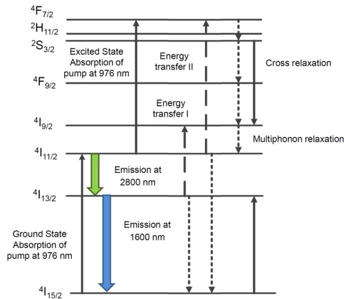
**Figure 6.** Scheme for the erbium doped fluoride fiber laser based on the cascade of the two transitions  $^4I_{11/2} \rightarrow ^4I_{13/2}$  at 2.8  $\mu\text{m}$  and  $^4I_{13/2} \rightarrow ^4I_{15/2}$  at 1.6  $\mu\text{m}$ . Figure adapted from [27].
