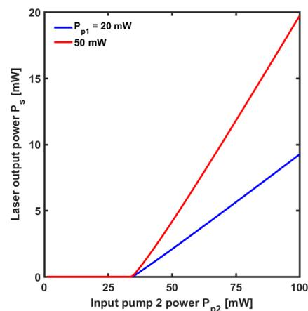
**Figure 10.** Characteristics of the dysprosium doped chalcogenide fiber laser pumped with quantum cascade lasers (QCLs). Figure adapted from [35].
