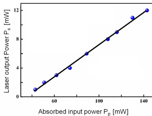
**Figure 2.** Characteristic of the  $\text{Nd}^{3+}/\text{Ho}^{3+}$  co-doped tungsten tellurite fiber laser. The blue points are measured. Figure adapted from [18].
