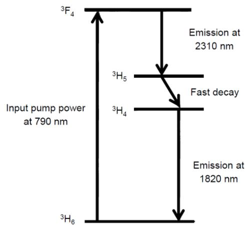
**Figure 3.**  $\text{Tm}^{3+}$  doped monomode fluoride fiber laser proposed in [21]. Figure adapted from [21].
