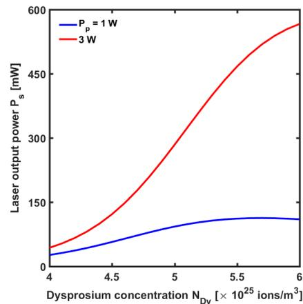
**Figure 9.** Characteristics of the dysprosium doped chalcogenide fiber laser based on the master oscillator power amplifier (MOPA) configuration. Figure adapted from [34].
