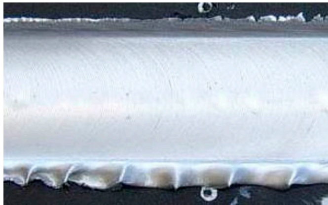
Figure 10. Surface of the joint which verified the best results in mechanical terms ( n = 500 rpm; v = 20 cm/min).
