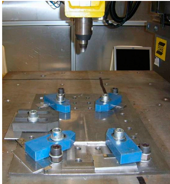
Figure 4. Positioning of the workpiece on the fixture table.
