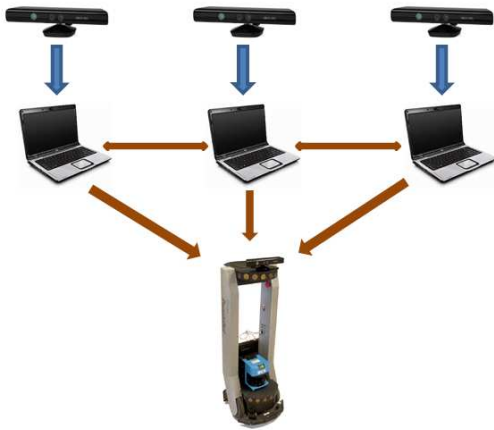
Figure 1. Scheme of the system architecture: the Kinects are connected to the computers which in turn wirelessly communicate with each other and with the mobile robot
