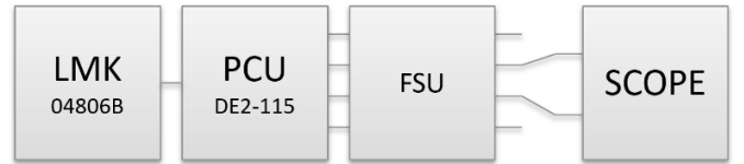
Fig. 9. Measurement setup employed during the qualification of the FSU outputs
