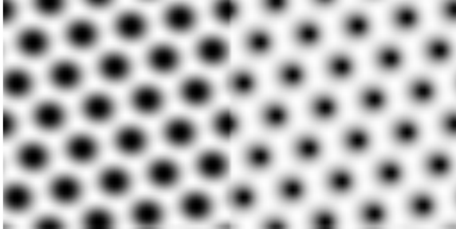
Fig. 3. (File size 1.71 MB) Movie showing the formation of a travelling honeycomb pattern in the transverse cross-section of the field intensity (left) and temperature (right), in the case of the passive configuration: integration window is about 140 \times 140 \mu\text{m} wide, while the evolution time is 24 \mu\text{s} . White corresponds to field intensity and temperature maxima. Temporal parameters are set as in Fig. 2. Other parameters are \Delta = -1 , \theta_0 = -6 , \alpha = 10 , Z \simeq 2.06 \cdot 10^{-3} , \Sigma = 40 , E_I = 15.5 .
