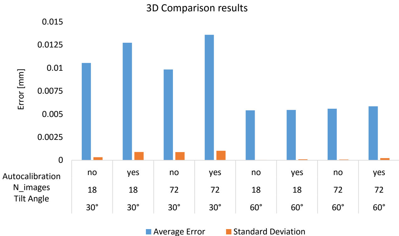
Figure 40 3D comparisons results: average error and standard deviation respect to the reference model obtained with Optimet Conoscan.
