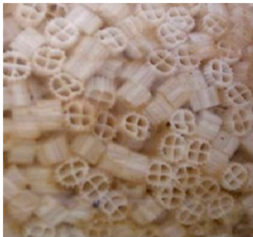
Fig. 2.5.2. Filling material kmt-k1 of Kaldnes.
