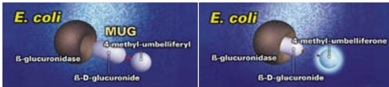
Fig. 2.5.6. E. coli use \beta -glucuronidase enzyme to metabolize MUG and create fluorescence (thermalindo.com).
