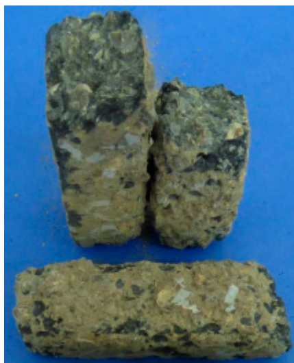
Figure 1. Conventional MgO-C bricks after usage. Source: LeanStory project.
