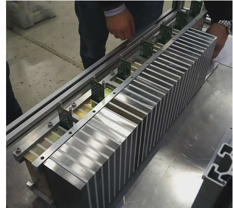
Figure 4. Photo of the calorimeter during the installation. The calorimeter is rotated by 90^\circ with respect to the layout.
