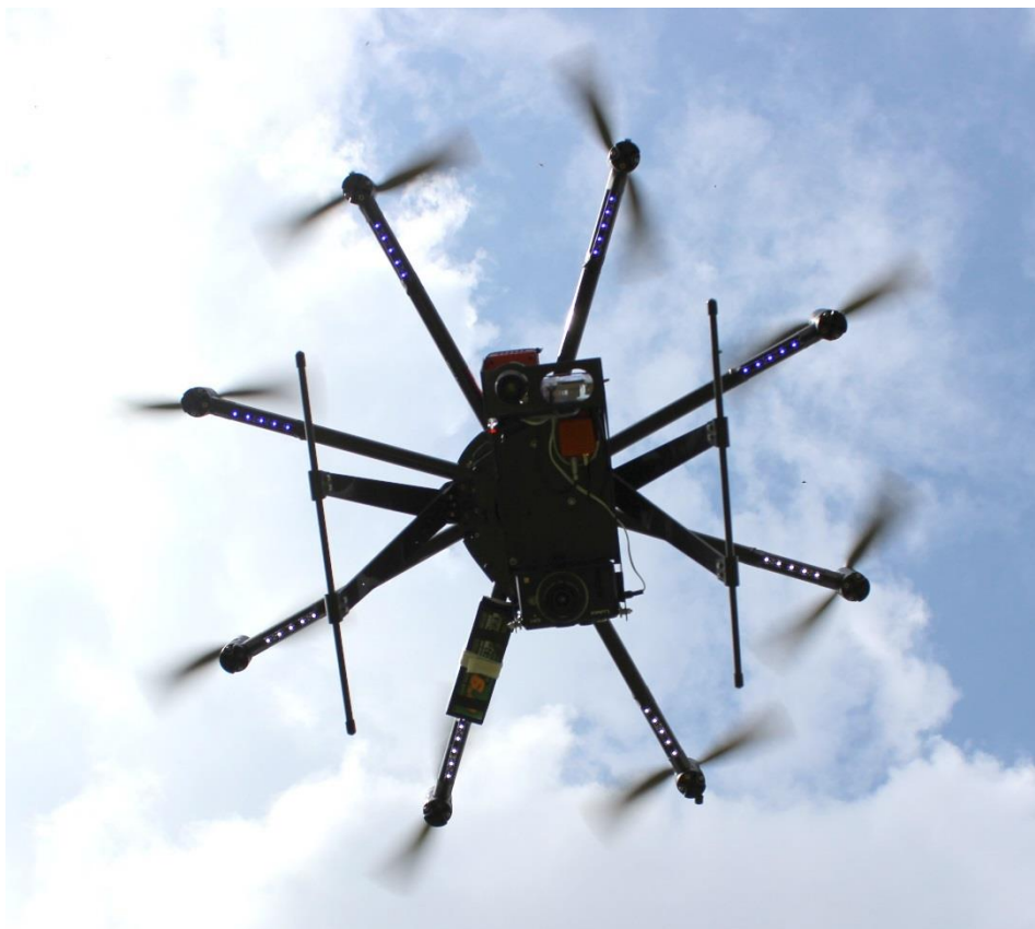
Figure 3. The octocopter UAV Aerialtronics Altura AT8 v1A equipped with all necessary hardware and software tools for its control and programming.
