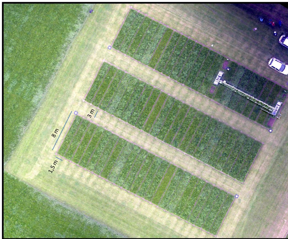
Figure 1. RGB ortho-mosaic of the experimental grassland plots on 15 May 2014, acquired using the Panasonic GX1 camera of the Wageningen UR Hyperspectral Mapping System (HYMSY).
