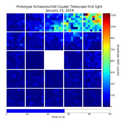
**Figure 3:** Skyward pointing view of first light from the pSCT. First light and first shower candidates were achieved on January 23, 2019. This is a snapshot of a single event. This data has not yet undergone any pedestal subtraction or data processing. The module in the center left is dark because it failed to connect.
