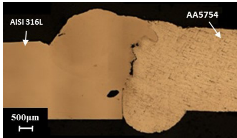
Fig. 79 Cross section by hybrid laser-MIG welding [155].
