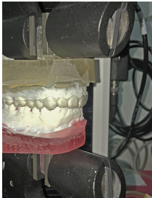
Figure 2.2.6. Resin models secured to the Instron machine.
