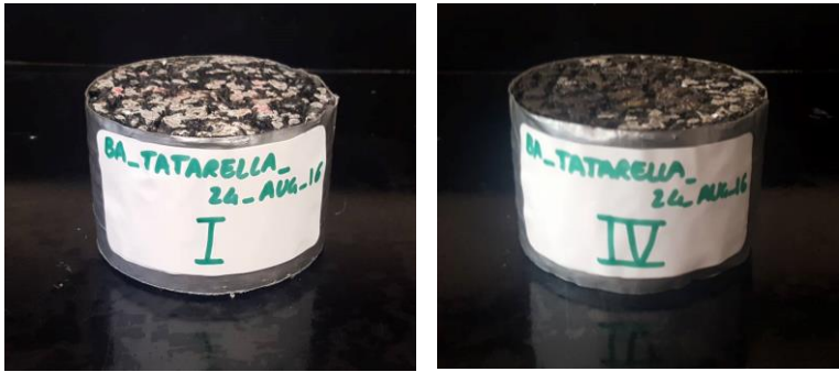
Figure 3-4 PA specimens (namely I and IV) cored from the permeable asphalt system located on the Adriatico Bridge.
