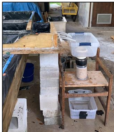
Figure 4-23 Picture ad-hoc self-developed device for filtration test on a combined system built in the laboratory.
