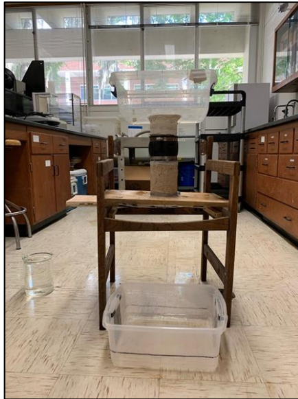
Figure 4-21 Picture of the ad-hoc self-developed device for the filtration test of the aggregates built in the laboratory.
