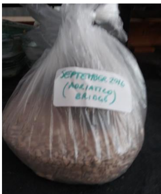
Figure 4-17 Coarse stone aggregates of the infiltration trench placed on the Adriatico Bridge (collected on September 2016, before the opening of the bridge).
