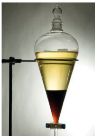
Figure II.12 - Separation of glycerine (bottom part) and FAMES (upper part).
