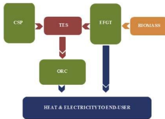
Fig. 1. Power blocks and energy flows through the proposed plant.
