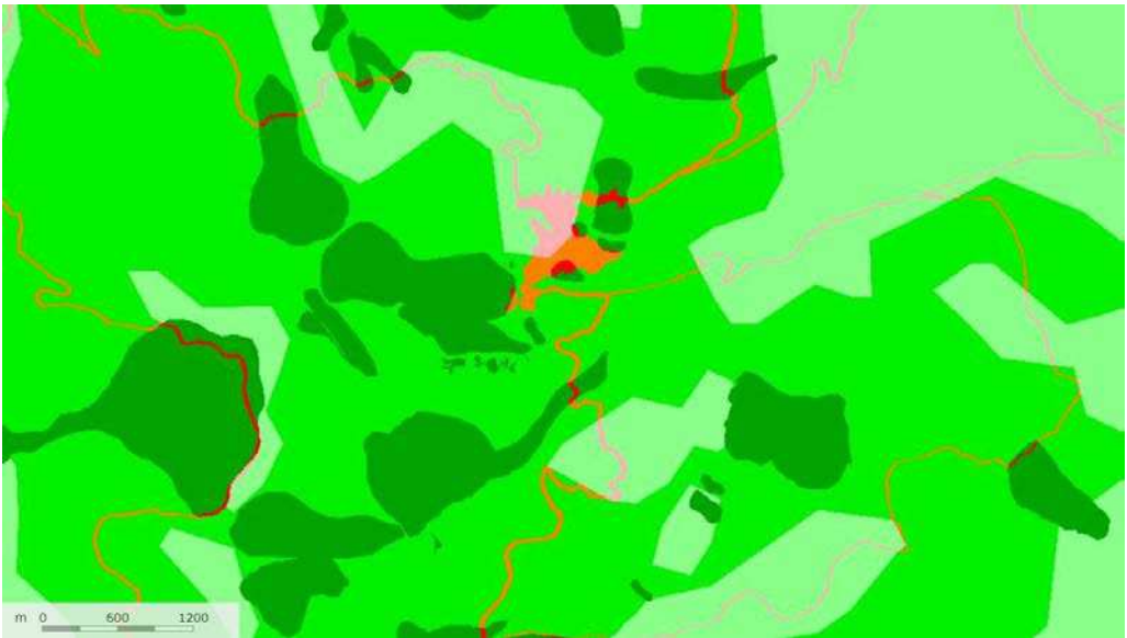
Fig. 36 - Landslide hazard and risk classes around the municipality of Deliceto, defined by the HSP of the Apulian Basin Authority.
