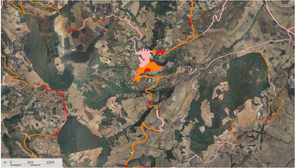
Fig. 35 - Landslide risk classes for the municipality of Deliceto and surrounding: R2 (rose), R3 (orange) and R4 (red), defined by the HSP of the Apulian Basin Authority.
