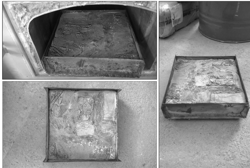
Figure 18 Obtained cast after melting and annealing phases.
