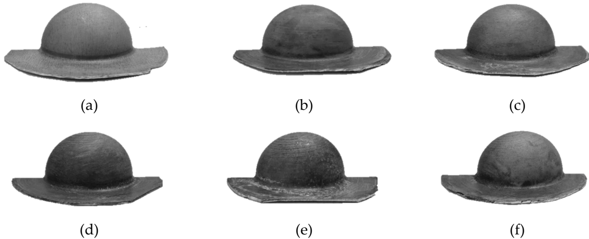
Figure 130: Sound samples obtained from experimental SPF tests. Samples from (a) to (c) were obtained starting from the SPIFed blanks with a SD of 0.2mm and a FR equal to (a) 200 mm·min -1 , (b) 400 mm·min -1 and (c) 600 mm·min -1 . Samples from (d) to (f) were obtained starting from the SPIFed blanks with a SD of 0.3mm and a FR equal to (e) 200mm·min -1 , (d) 400mm·min -1 and (f) 600mm·min -1 .
