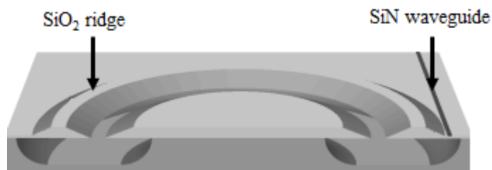
Fig. 2.5. \text{SiO}_2 wedge resonator and a SiN waveguide as bus [57].
