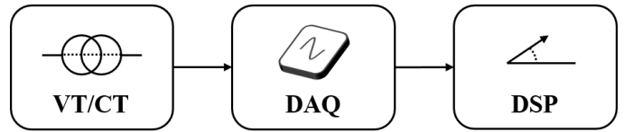
Fig. 1. PMU signal chain: voltage/current transformer (left), synchronized data acquisition system (center) and phasor estimation (right)
