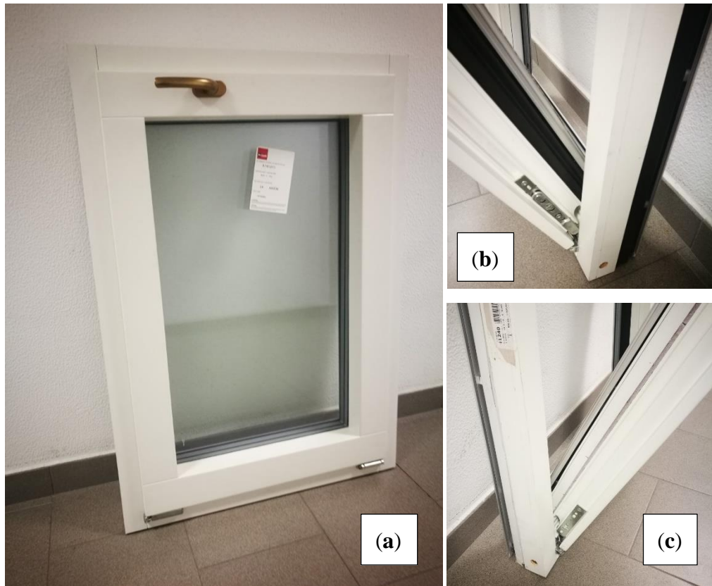
Figure 3. Aerogel-enhanced window (Aeroshield) embodying a triple-glazed unit, with external aluminium frame and internal wooden frame (a); Reference frame with expanded polystyrene insulation, in black (b); Aerogel-insulated frame with polymer skin (c).
