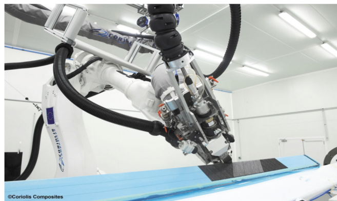
Fig. 1. Coriolis ® robotic system equipped with a roller of the Robotic system, Denkena (2016).
