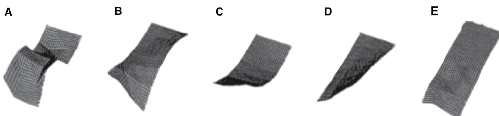
Figure 4: Different resonance modes by modal analysis (no hole specimen). (A) First mode (B) second mode (C) third mode (D) fourth mode (E) fifth mode.
