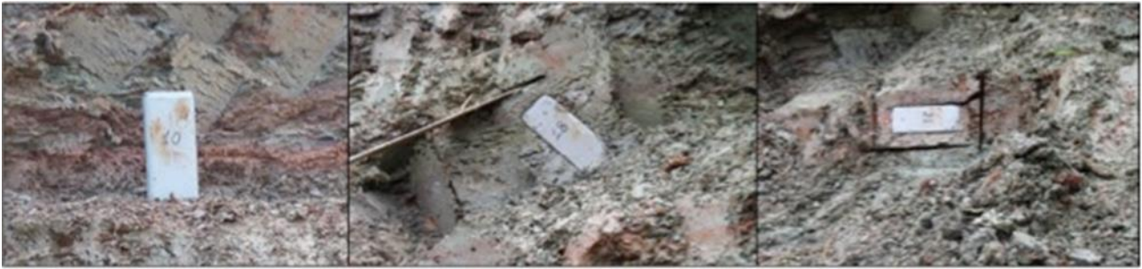
Fig. 1. Sampling by means of the C-shaped steel samplers. They were inserted in-situ with three different orientations.
